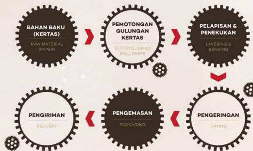
horizontally with glue. The process followed by laminating layer of honeycomb become honeycomb board. After passed drying process, honeycomb board is ready to be packaged and delivered to customers.
